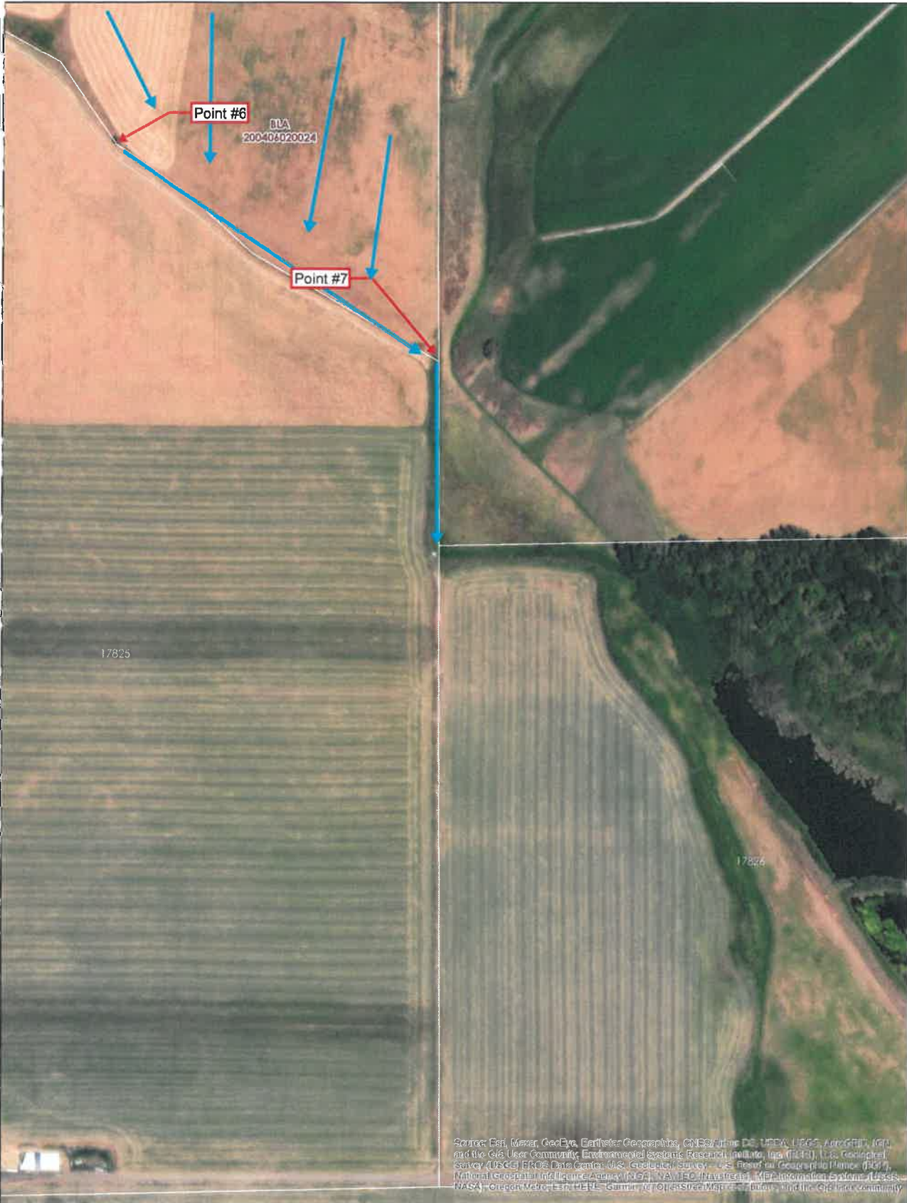
Figure 3.1 - Downstream Analysis Flowpath
